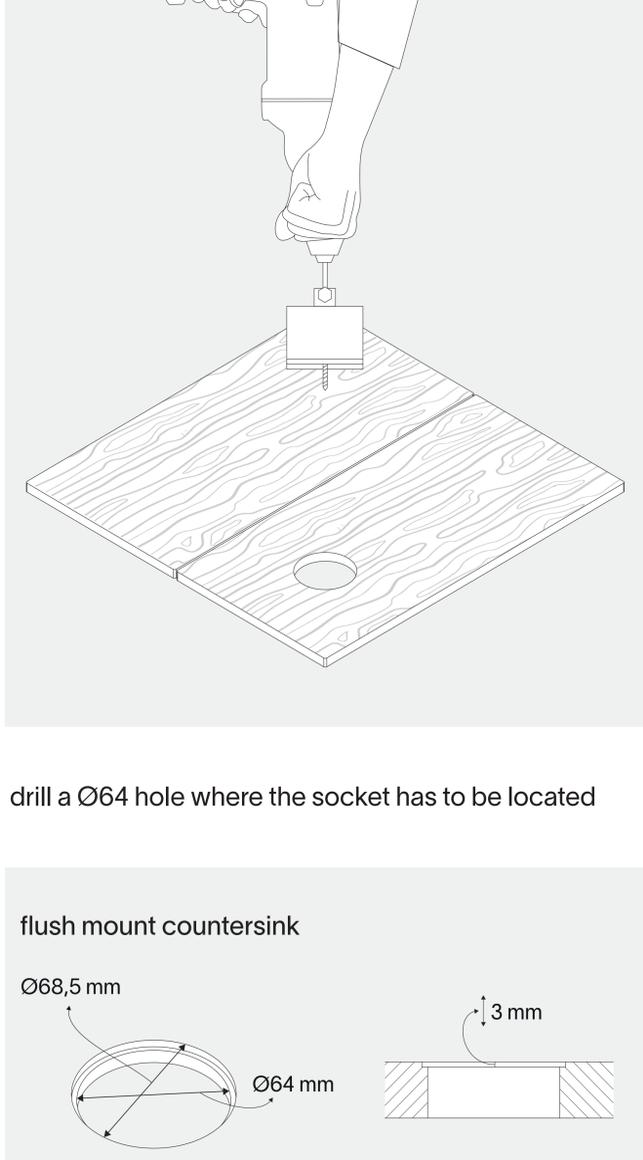
drill a Ø64 hole where the socket has to be located
