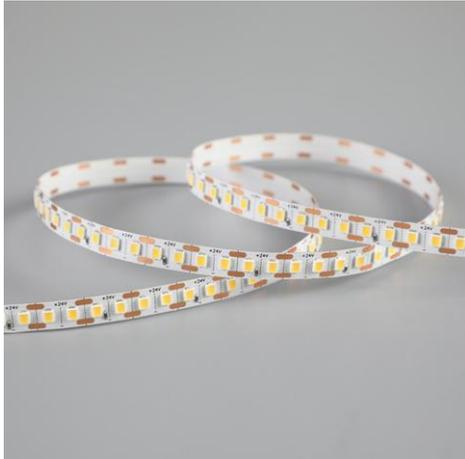
LED strip from the PERFORMANCE series. The strip is distinguished by a high CRI and consists of 160 SMD LEDs per meter and has an energy class E. Suitable for indoor, dry environments: IP20. Roll of 5m. Power of 10,5W/m. The led strip is controlled with a voltage of 24Vdc. The strip delivers 1250 Lm/m and has a color temperature of 3000K at a CRI of 95. The strip is dimmable via PWM.
